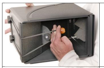
For shipping and storage, place the removable mirror against the beam splitter to protect both. (Beam splitter measurement is 349mm x 157mm x 3mm)
