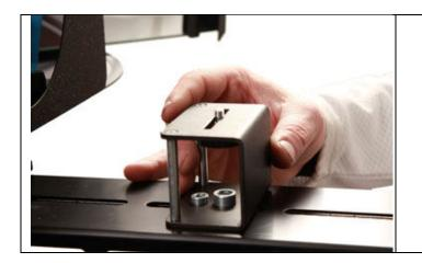
The base plate has slots that assist front to back adjustments.
