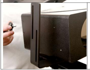
Attach the mirror box with 1/2 inch 1/4x20 tie down knobs (included).
